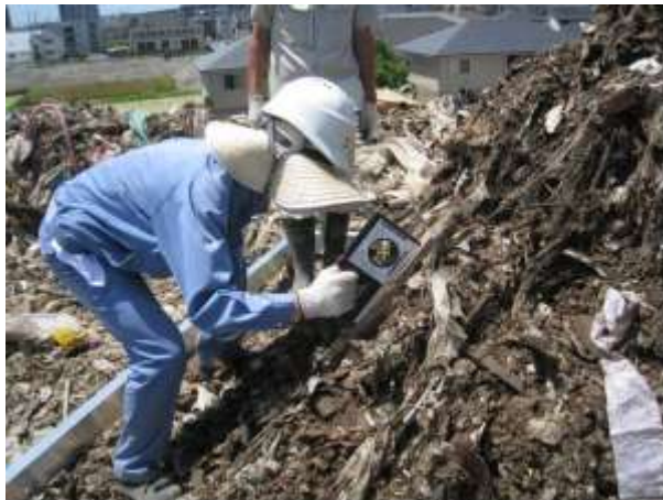
Measuring slope angle
