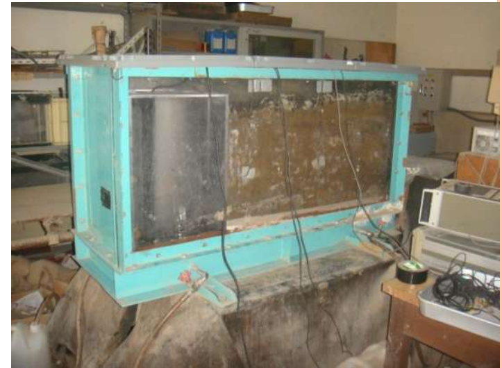
The situation of shaking table test
