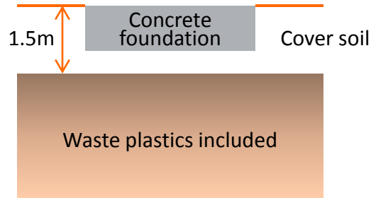
Concrete foundation on a landfill in Chubu district (7m in diameter, 1m thick)
