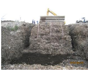
Photograph 2. Loading test (Shanghai Site) (Slope stable even though safety factor was 0.56 by conventional assessment)
