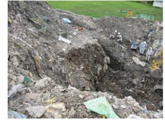
Photograph 4. After collapse (Failed at 40°)
